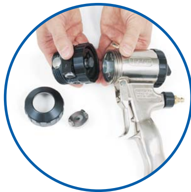
Remove the fluid section from the gun
